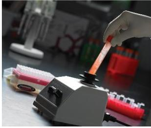
The Corning variable speed LSE Vortex Mixer provides fast, efficient mixing with minimal vibration. The unit features a powerful, counter-balanced motor drive, continuous or mix modes. A range of accessories are available for all common sample tubes and containers.
