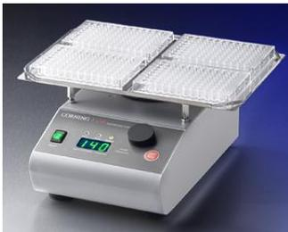
The Corning LSE Digital Microplate Shaker features digital control of shaking speed and run time. A single control knob is used to set parameters, and values are shown on a large 3-digit display. A sturdy base encloses the motor for quiet, vibration-free operation. The included stainless steel platform accommodates up to 4 microplates (standard or deep well) and the shaker is safe for use in temperature controlled environments from 4 to 65°C.
