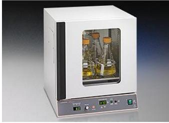
This cabinet-style incubator has a compact footprint and can also be stacked to maximize space efficiency. The built in orbital shaker accepts a large assortment of platforms and clamps that can accommodate flasks, Petri dishes, and test tube racks. The maximum capacity is 4 x 1L flasks.
